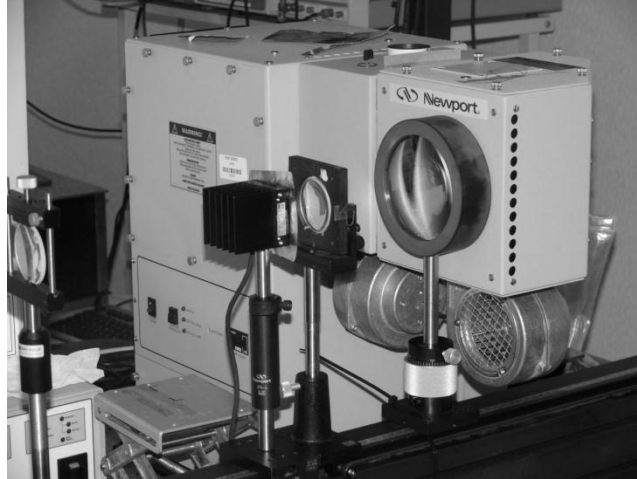
Figure 6. AFIT Xenon Thermal Simulator
