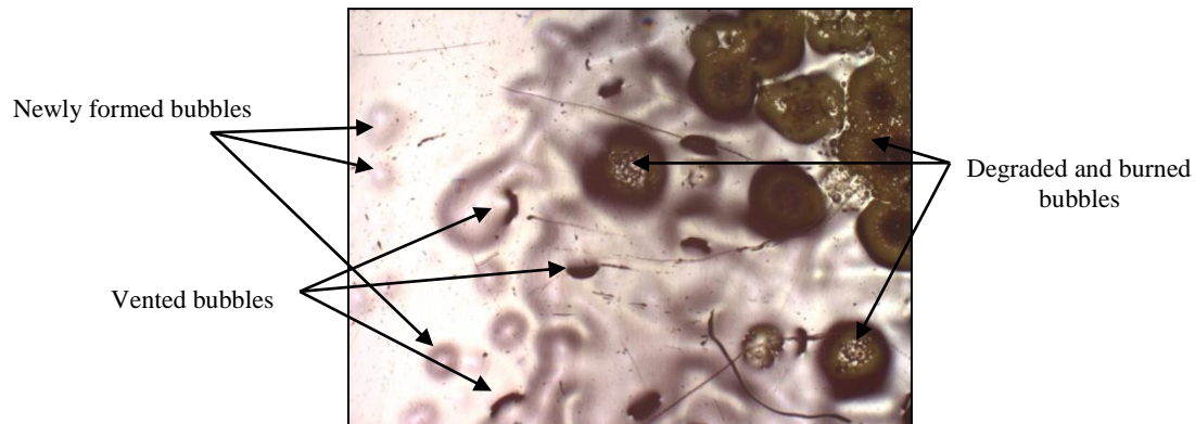
Figure 27. Paint sample showing stages of thermal degradation
